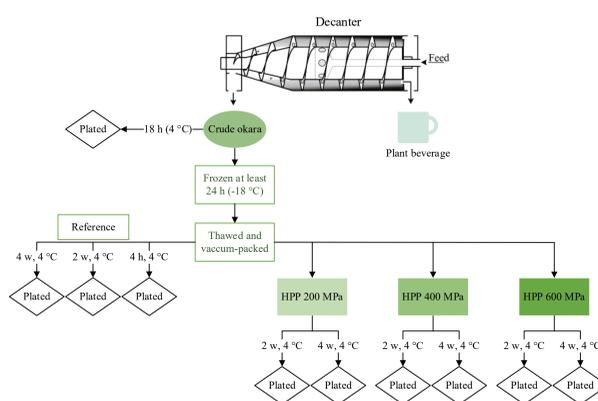
Fig 2. The storage study schedule for the high-pressure pasteurization study.
