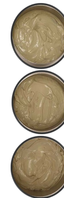
FIGURE 3. Precipitates from time trials, 1 h (top), 2 h (middle), 3 h (below).
